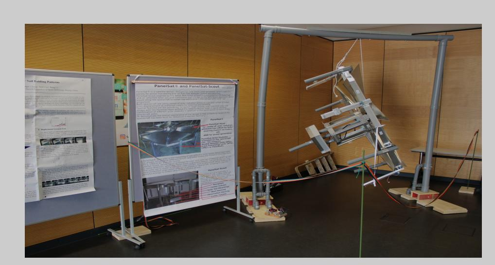
bulky, manually constructed 1.8 m model. It couldn't orient itself, and the motors weren't strong enough to move the panels, when pointing towards earth center.
