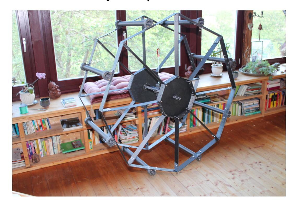
Suspending the PanelSat® model from a thread revealed an important behavior. it did self-align.
